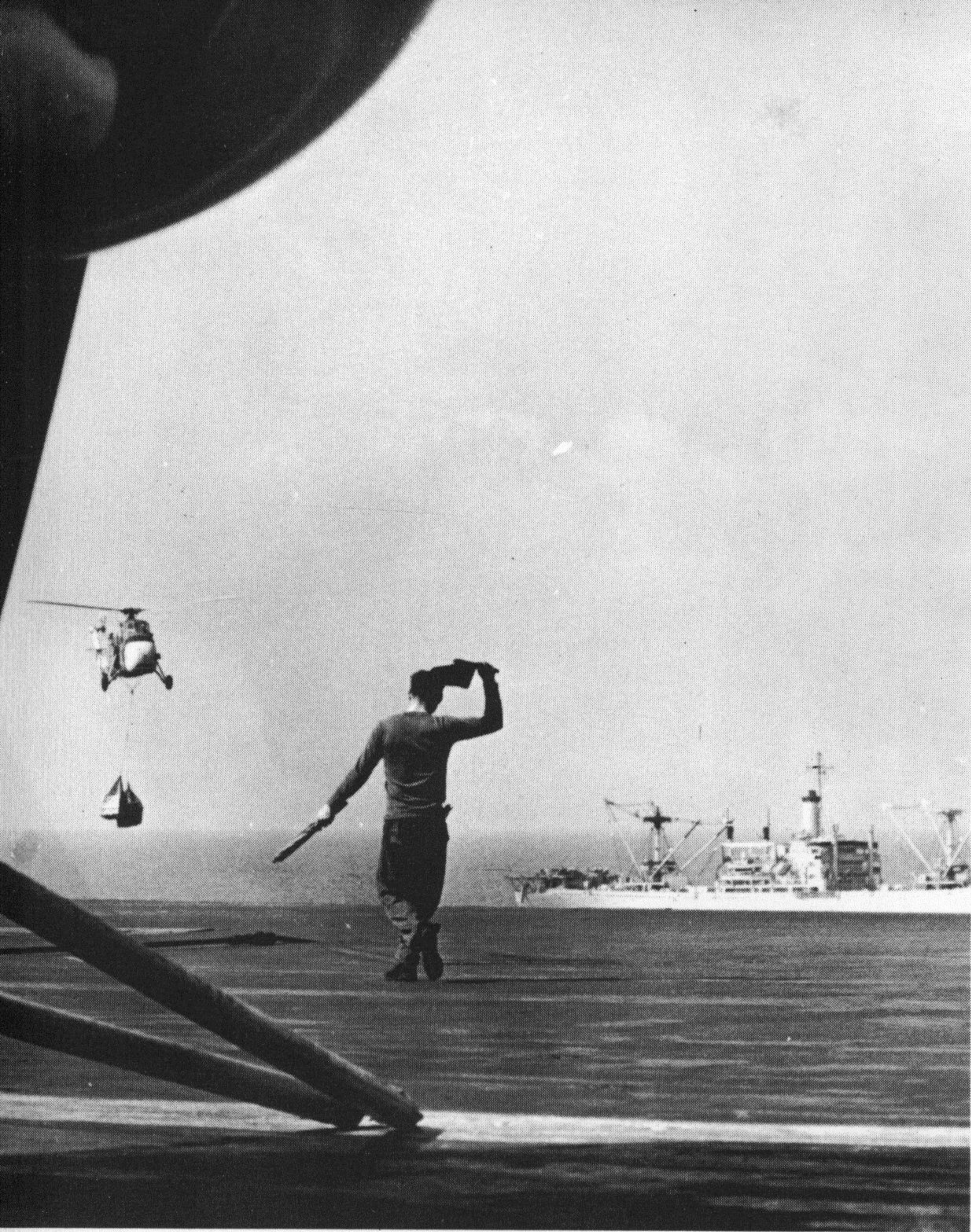
Helos lift cargo from the supply ship's small flight deck and helo-haul it to the flight deck on the ENTERPRISE.
