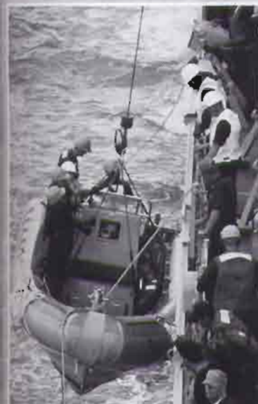
The SLAD drops the RHIB into the water while First Division keeps the fore and aft lines tight.
