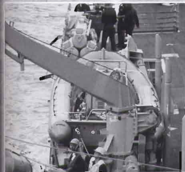
BM3 Morehouse controls the movement of the SLAD while the RHIB is put back into its skid, SN Kimball is the SLAD controller.
